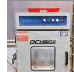
Battery Explosion-proof Testing Chamber
