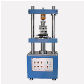
Charger Plugging/ Unplugging Tester
