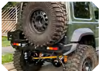
UNI-JN18-RB03 SUZUKI JIMNY 2018+ Rear bumper (with Jerry can holder+Spare tire carrier)
