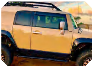
UNI-SSFJD Toyota FJ Cruiser Side Step Material:Steel Plate:3.0MM step Bar:1.5MM
