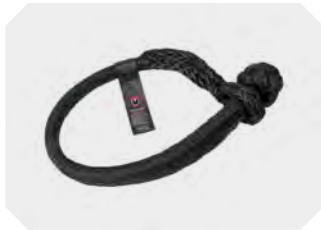
Soft Shackle Incredible 21.3t (47,000lb) rated breaking strength Made from High Modulus Polyethylene (HMPE) 12 - strand synthetic rope One - piece construction is quick to fit and requires no pin - fastening
