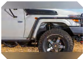
UNI-SSLC79 Toyota LC79 Side Step 2007+ With Bush Bar
