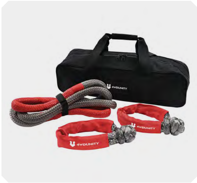
Snatch Straps Minimum Breaking Strain 12000kg, 10cm x 9metre with 20% elongation , the kinetic energy generated by the elasticity aids with the recovery itself, while at the same time reducing the likelihood of vehicle damage
