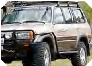
UNI-SSLC80 Toyota LC80 Side Step With Bush Bar Material: Steel Plate:3.0MM step Bar:1.5MM
