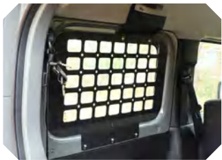
UNI-JN18-ER Aluminum alloy expansion frame inside window for JIMNY (JB64/JB74) 2018+
