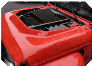
UNI-JLJG-02 Jeep Wrangler JL Sandstorm Hood Material: Fiberglass
