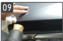
09 Edging with baking gun to get better effect.
