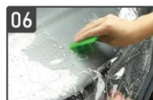
06 Use the scraper to push out the blisters under the protective film.
