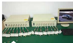
Battery capacity aging tester
