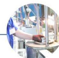
Welding bottom 焊底
