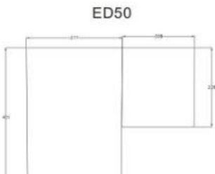
冷冻/冷藏区(Freezer/Refrigerator compartment) L312*W277*D405(mm) 冷冻/冷藏区(Freezer/Refrigerator compartment) L312*W203*D235(mm)
